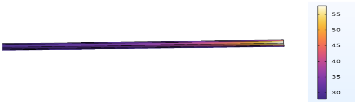
Figure 41: Temperature contour in PVC pipeline
