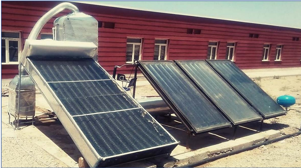
Figure 26: An illustration of the Iranian-made humidification-dehumidification desalination system [42].
