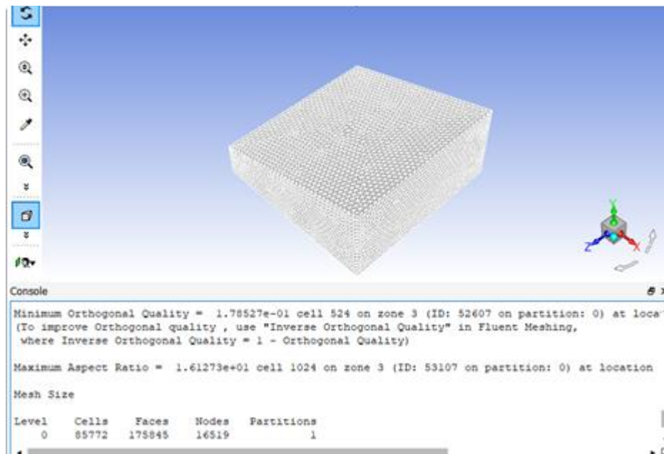
Figure 2, Orthogonal Quality of Meshes.
